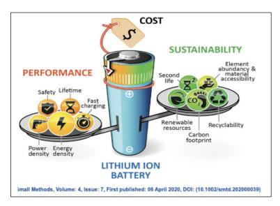
The request of the European Commission to produce no CO2 in 2050 is pushing the electrical transition. It is so clear the need of storage systems. Li-ion batteries are one of the main electrochemical storage systems actually used ad they allow the highest level of energy density. Performances such as fast charge or temperature operating window (-50°C up to 125°C) can be fine-tuned by the large choice of cell design and chemistries.
