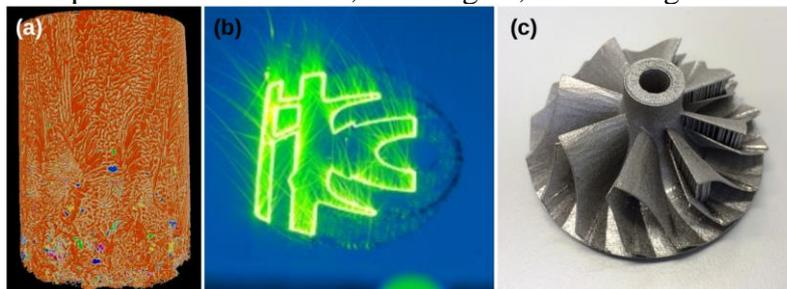
**Figure 1:** (a) 3D rendering of the Ti-32.5wt%Fe obtained by NF-PCXT [2]. (b) Rocket engine components being produced by selective laser melting. (c) 3D printed compressor wheel. Figures from: [www.dlr.de/wf/en](http://www.dlr.de/wf/en)
