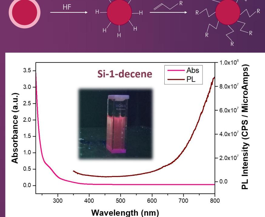
with SiNCs various surface functionalities, in particular 1-decene 1-octadecene, and were prepared by wet chemistry. A significant enhancement of the photoluminescence efficiency is observed.
