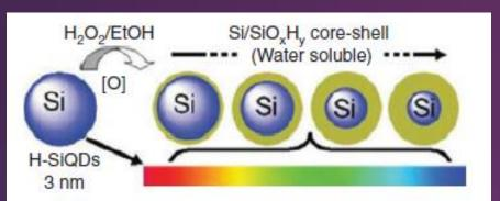
The optical emission properties are determined by a very complex interplay between the size dependent quantum confinement effect and the surface properties.
