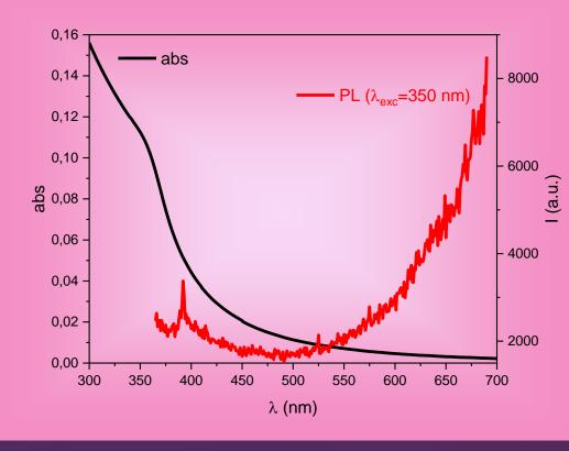
Produced Si nanoparticles have a crystalline core, covered by an oxide layer, with hydrogenated surfaces, and estimated average diameter 13.0 nm, but with a good part of nanoparticles under 10 nm. They show very low luminescence.
