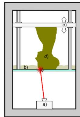
**Stereolithography** - A light-emitting device a) selectively illuminate the bottom of a tank b) filled with a liquid photo-polymerizing resin; the solidified resin d) is progressively dragged up by a lifting platform e). Adapted from Scopigno et al, DOI:10.1111/cqf.12781.
